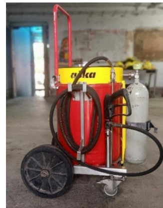
Pic 3.5: Trolley mounted Foam Drum
